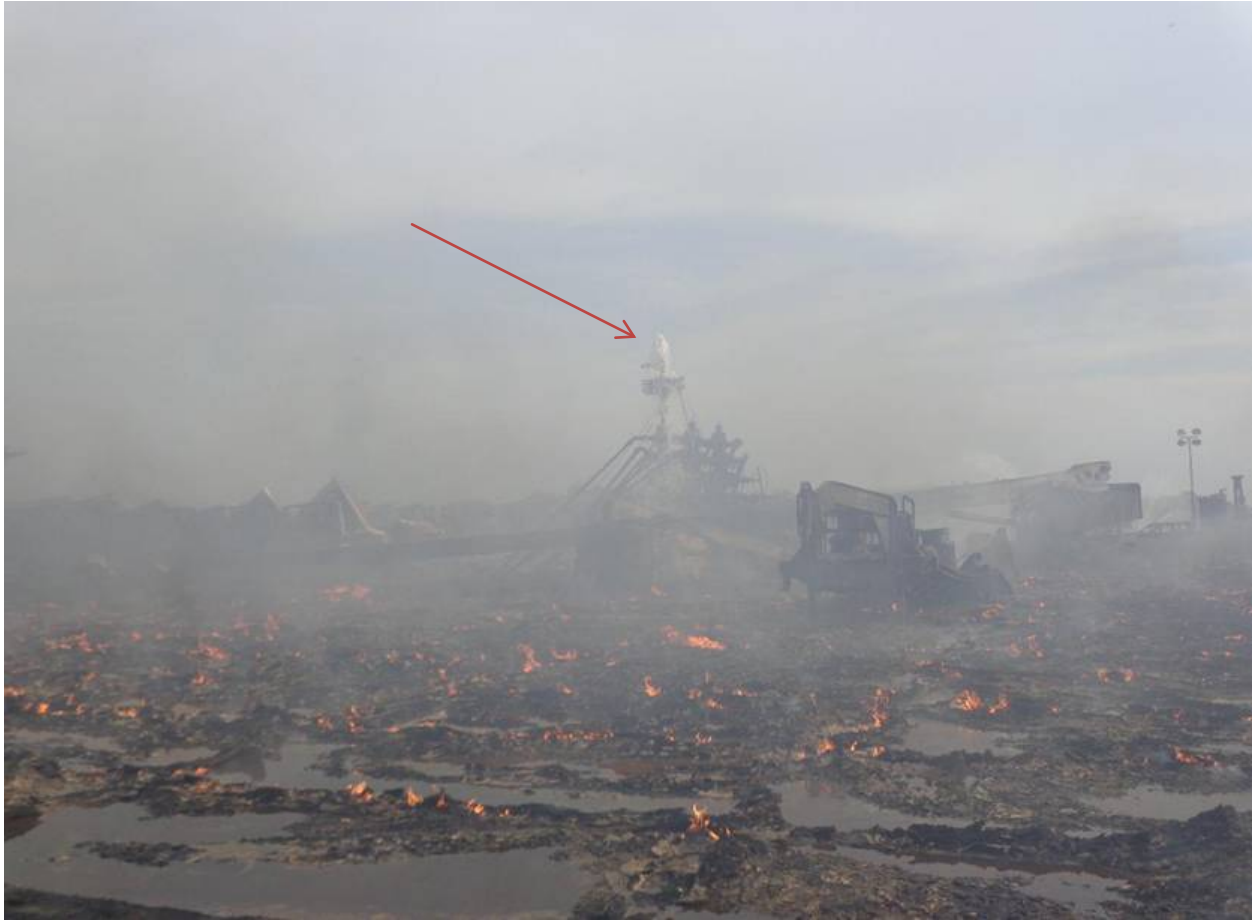
Monroe County well pad chemical fire. Note the flowback fluid coming back out the top of the frack stack.
