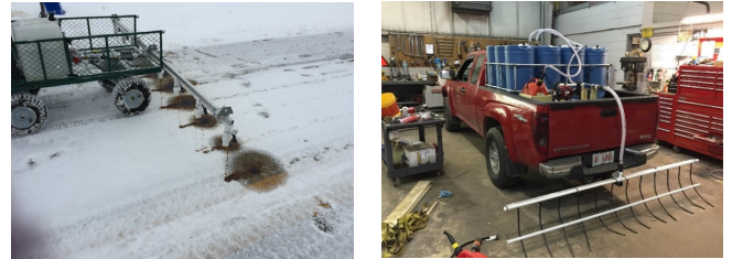
Figure 3: Application Systems (left is for no volume and right is form low/medium volume application)
