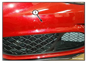
2. Release the coverfrom the facia by pulling the tether(1) from the retainer.
