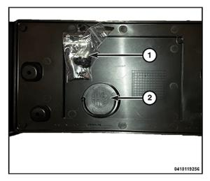
4. Align the license plate bracket (1) onto the front fascia by aligning the protrusion on the back of the bracket with the alignment hole on the fascia.
