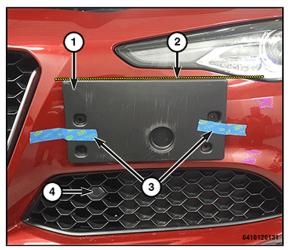
8. Attach the license plate bracket to the fascia by securing it using the four supplied self-tapping screws.
