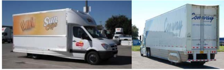
Figure 12. Examples of aerodynamic side skirts that could also provide side underrun protection.
