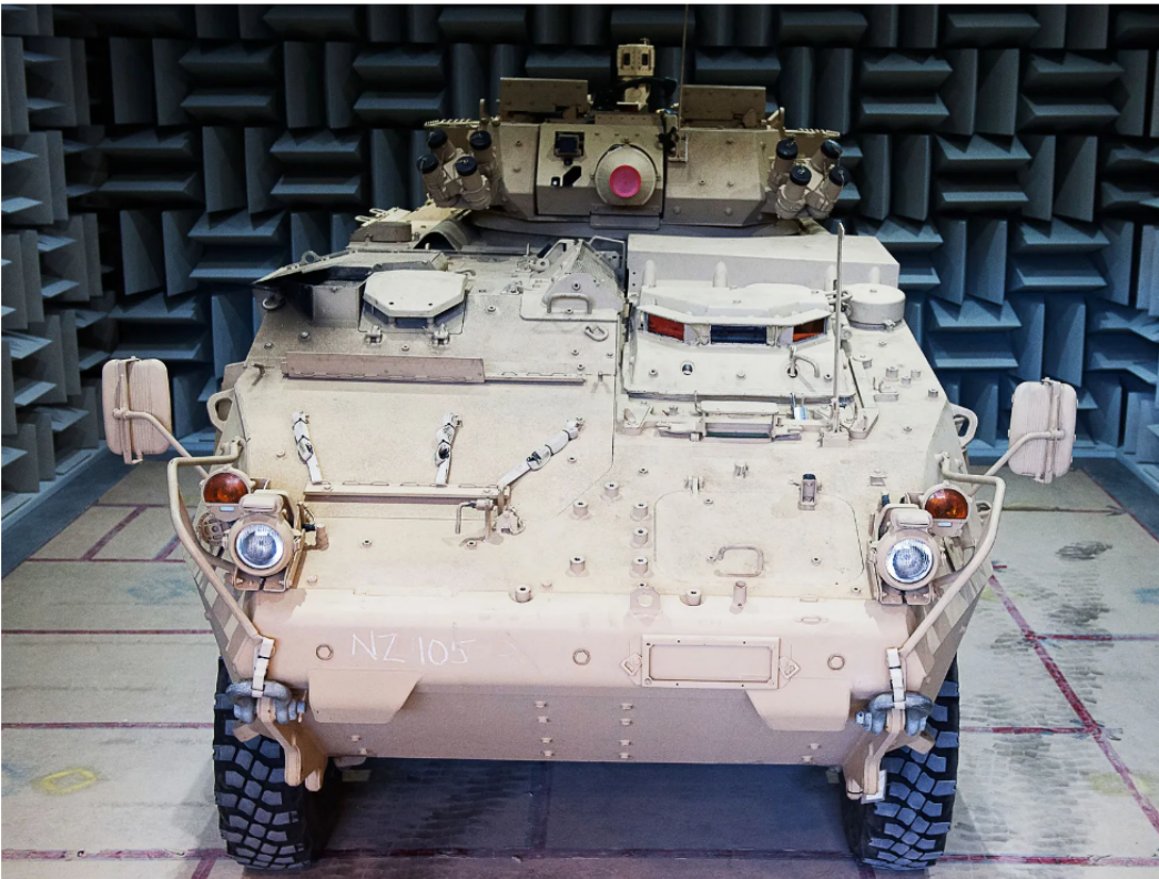
The anechoic chamber can also assess the acoustic properties of vehicles and research strategies for helping occupants better process incoming sounds on the battlefield. ECKEL NOISE CONTROL TECHNOLOGIES
